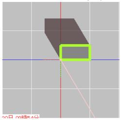
The clicked surface is highlighted with bold lines as shown above and set as [PV placement plane]. Clicking the highlighted surface again deselects [PV placement plane].
