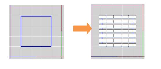
(d) Click the inner side of PV placing area. Then the PV arrays are placed automatically.
