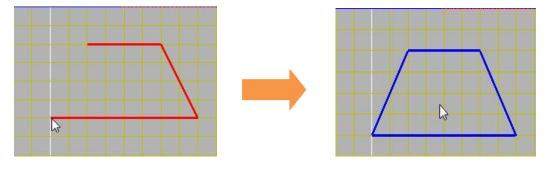
(5) Click the [Solid generation (Boundary line)] icon <sup>(1)</sup> on 3D model tool bar. Then, [Solid gen.(Boundary line)] command toolbar will be displayed.
