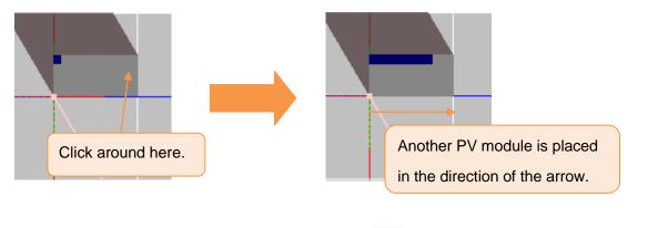
After placing all PV modules, click the [Cancel] icon above the 3D drawing to terminate the
