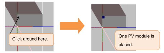
6 Click another location in the PV placement plane. Another PV module is placed in the direction of the clicked location from the PV module that has been already placed.
