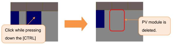
After deleting the PV module, click the [Cancel] icon above the 3D drawing to terminate the [Place PV module or Release PV module] mode.
