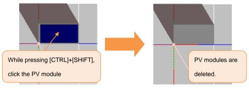
(5) Click the [Cancel] icon eabove the 3D drawing to terminate the [Place PV module or Release PV module] mode.
